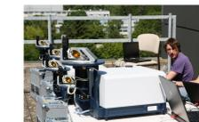
Side-by-side intercomparison of COCCON spectrometers, open path measurements
