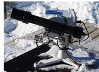
Testing of a fiber-coupled IR-Cube FTIR spectrometer.
