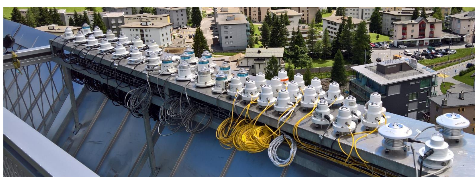
Figure 6. PMOD/WRC Roof Platform for the absolute calibration relative to the Qasume reference spectroradiometer [3].
