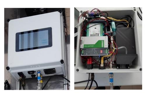
Both system, old HPP monitoring boxes and new AtmoBox, have a 4G modem to send automatically the data daily. They are also equipped with controlled (by sequencer) 3 ways solenoid valves in order to measure regularly calibration and/or QC cylinders. At least, one cylinder is measured daily (in afternoon) to correct the short term variability. Due to safety rules, the cylinder and Sensor boxes are enclosed in a vented, weatherproof casing.
