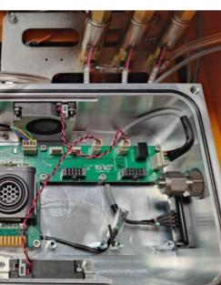
Cell equipped with a K96 Sensor (mounted on daugther board)
