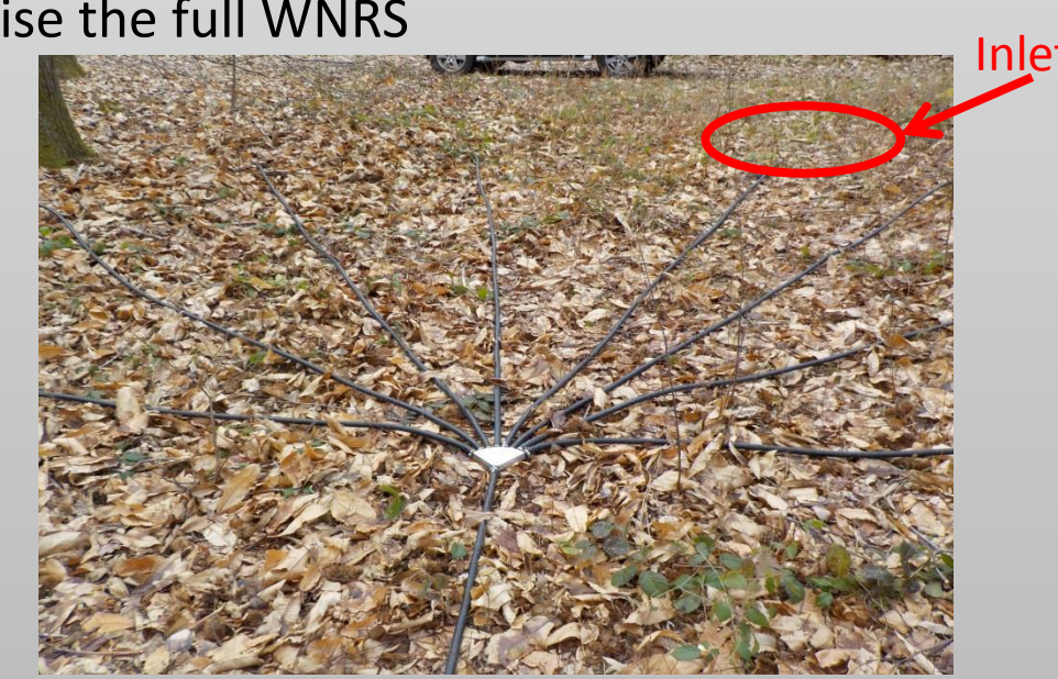
Single rosette with 8 inlets. 4 similar rosettes comprise the full WNRS
