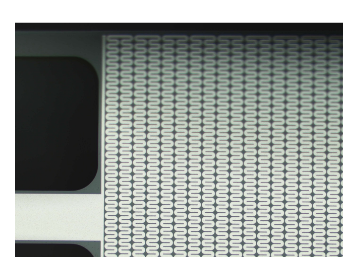
Metal traces on SiN Membrane
